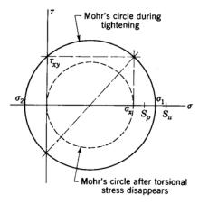
Fig. 7-17 Mohr's circle diagram for a bolt during tightening. Torquing of the nut produces shear stress  $\tau_{xy}$ . The bolt tensile stress is  $\sigma_x$ . The proof strength is  $S_p$ , and the tensile strength  $S_u$ .
