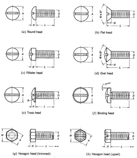
Fig. 7-9 Types of heads used on machine screws.
