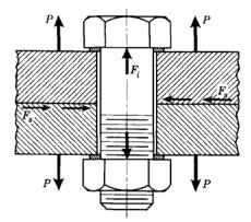
Fig. 7-12 A bolted connection.
