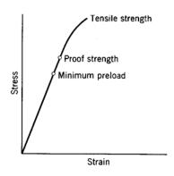
Fig. 7-16 Typical stress-strain diagram for good bolt materials.
