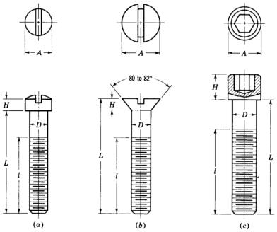
Fig. 7.10 Cap-screw heads; (a) Fillister head, (b) flat head, (c) hexagon socket head.
