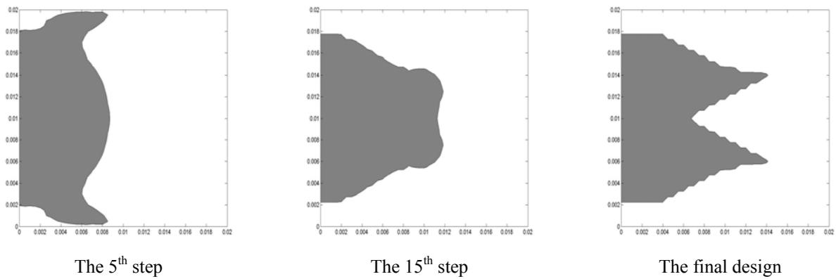
Figure 3: The intermediate and optimal topology of the sensor
