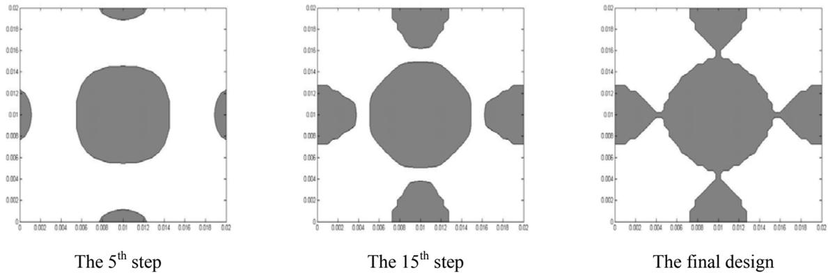
Figure 5: The intermediate and optimal topology of the sensor
