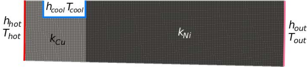
Figure 3: Schematic of a regeneratively cooled rocket engine combustion chamber. The drawings are not to scale.
