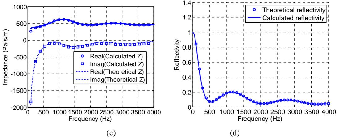
Figure 2: Pressure attenuation of a layer of a fibrous material of thickness  $d$  with the normal flow resistivity equal to  $10000 \text{ Nm}^{-4} \text{ s}$ . (a) A schematic layout to measure the absorptivity and the impedance, (b) the employed finite element model and the sommerfed boundary condition for the sound source, (c) the complex impedance  $Z$  calculated by (6) and the present approach and (d) the normal incidence reflectivity from the uniform fibrous layer.
