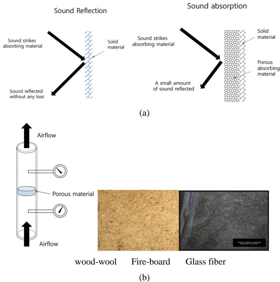
Figure 1: Examples and applications of absorptive porous materials. (a) A comparison of the reflected sounds by a solid (rigid) wall versus an absorptive wall, and (b) examples of porous materials and a drawing of the impedance tube method, used to measure the bulk acoustic properties of the porous materials
