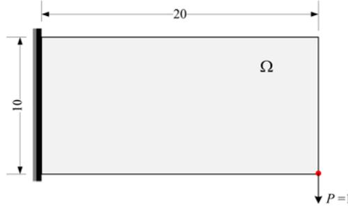
Figure 1: Design domain and boundary conditions for the cantilever beam problem
