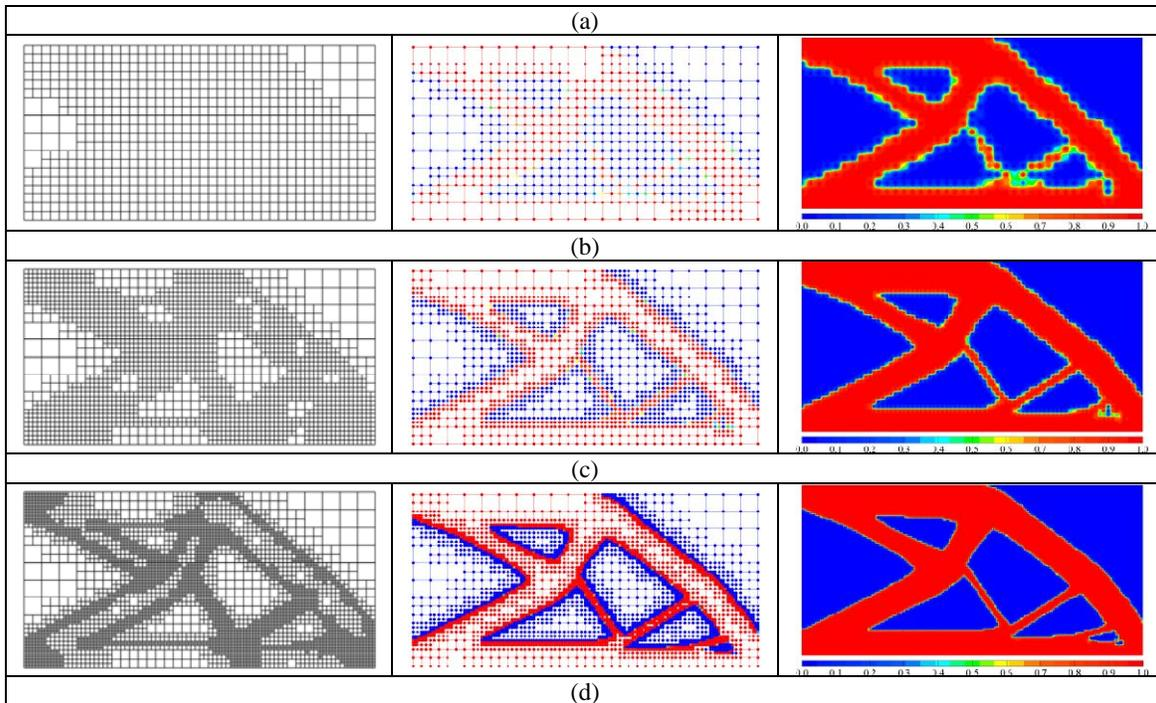
Figure 2: Optimization results under each refinement level
