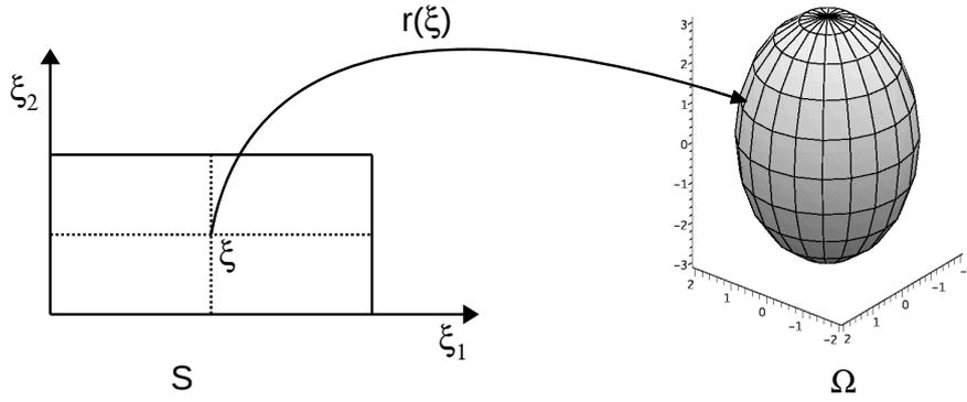
Figure 2: Cavity shape parametrization.
