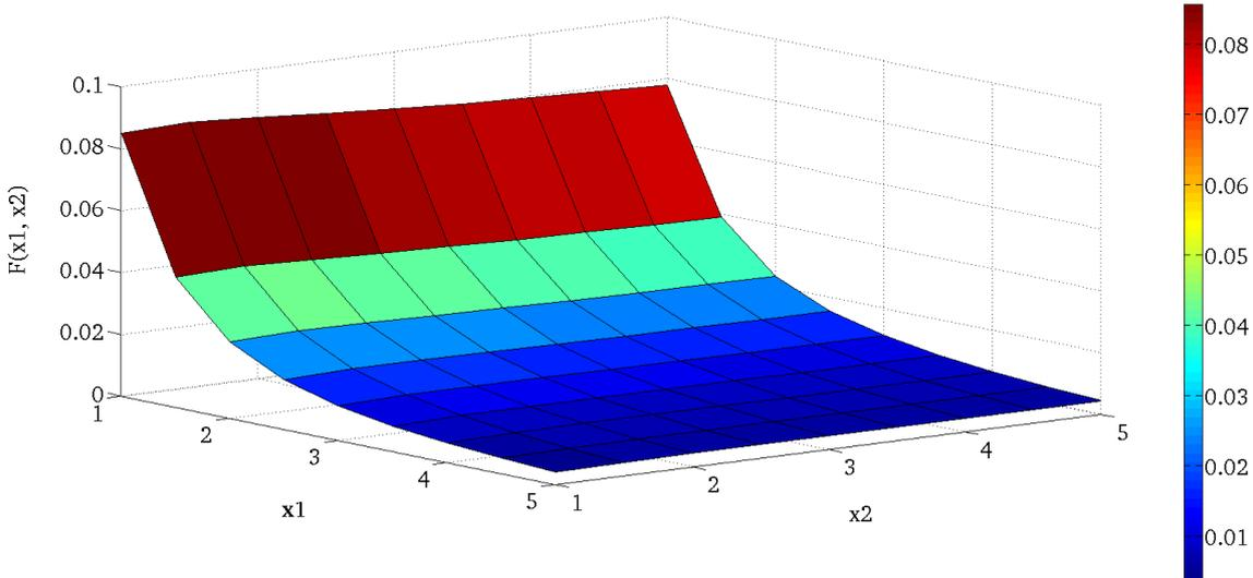
Figure 3: The norm of energy density vector  $\| W \|$  as function of design variables  $x_1$  and  $x_2$ .
