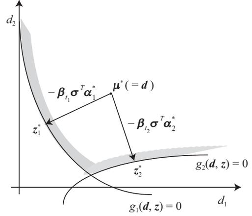
Figure 2: Relation between variables in applying SLSV.
