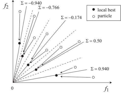
Figure 4: Global guide selection by sigma method
