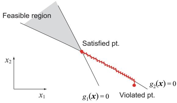
Figure 1: Feasible domain and example of moving paths to feasible boundary.
