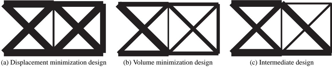
Figure 12: Typical Pareto optimum configurations of 10-bar truss.
