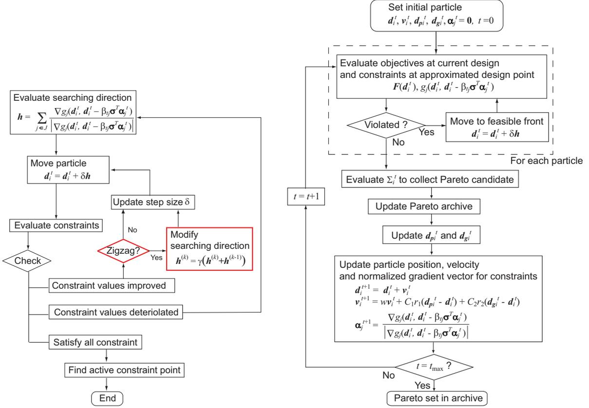
(a) Constraint satisfaction with eliminating zigzag iteration. (b) Reliability-based multiobjective optimization.
