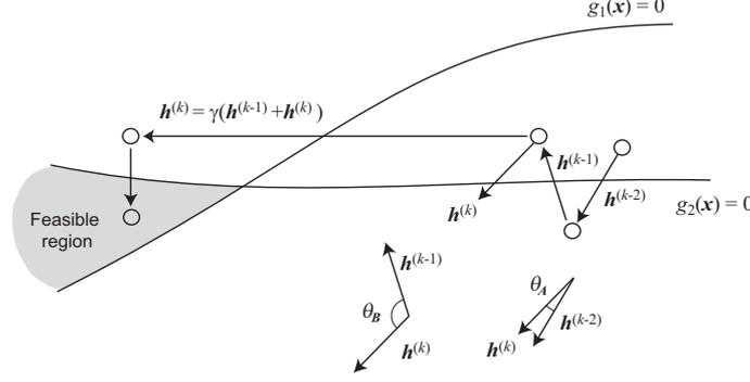
Figure 5: Image of zigzag elimination
