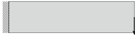
Figure 4: The design domain, boundary conditions, and external load for the optimization of cantilever
