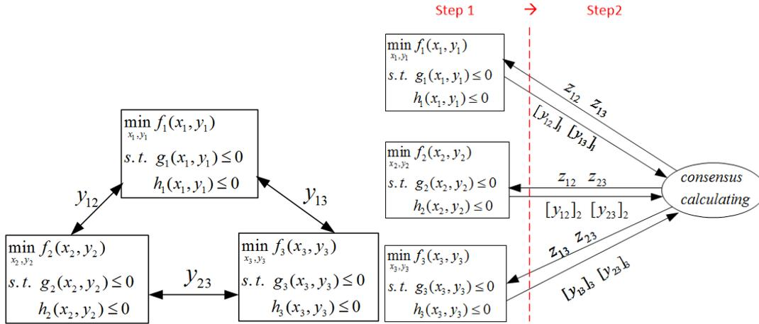
Figure 2: Original problem (left) and decoupled problem (right) for CADMM
