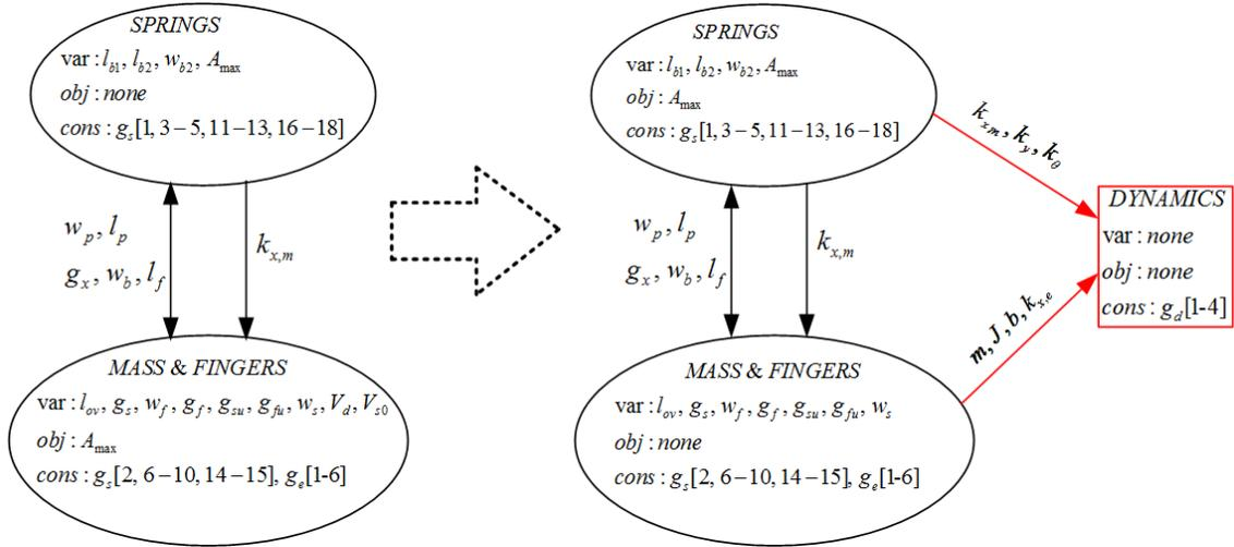
Figure 4: Hybrid decomposition 1 for the micro-accelerometer problem
