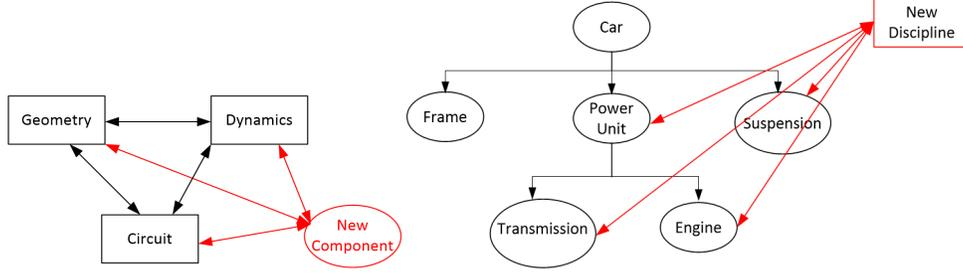
Figure 1: top left - discipline-based decomposition; top right – component based decomposition; bottom – hybrid decompositions (rectangle stands for discipline, circle stands for component )
