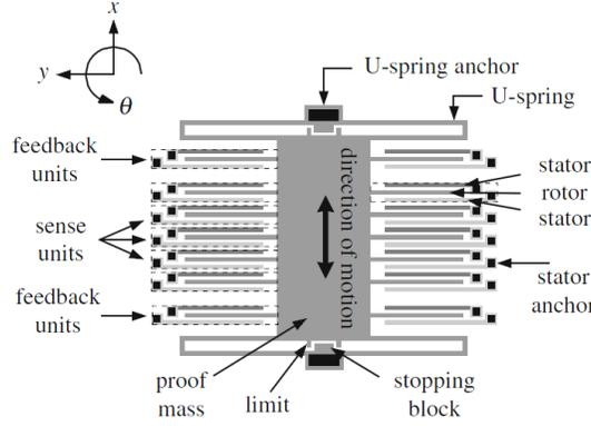
Figure 3: Schematic illustration of micro-accelerometer design [10]
