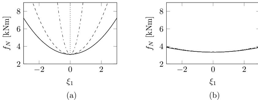
Figure 4: Clamped column: performance as a function of the first mode of imperfection for (a) the nominal design and (b) the robust design: normalized linear compliance (full line) and nonlinear end-compliance for load levels  $\lambda = 40\%$  (dashed line),  $\lambda = 80\%$  (dash-dotted line) and  $\lambda = 120\%$  (dotted line).
