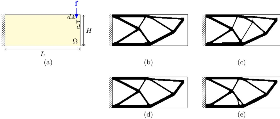
Figure 5: Cantilever design: (a) design domain and boundary conditions, (b) linear nominal design, (c) linear robust design, (d) nonlinear nominal design and (e) nonlinear robust design.
