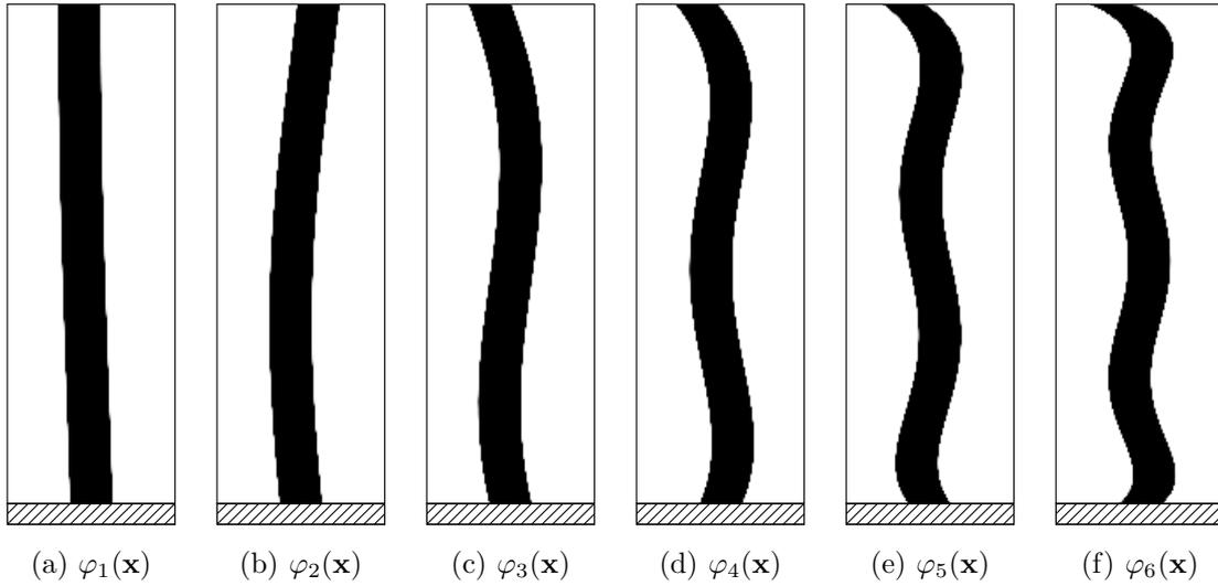
Figure 3: Modes of the EOLE expansion of the Gaussian random field  $\mathbf{p}(\mathbf{x}, \theta)$  applied to the nominal column design. The modes  $\varphi(\mathbf{x})$  are normalized and multiplied by a constant factor = 80 in order to show the difference in mode shape.
