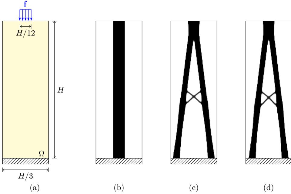
Figure 2: Clamped column: (a) design domain and boundary conditions, (b) nominal design, (c) linear robust design and (d) nonlinear robust design.
