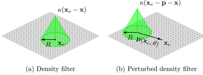
Figure 1: Translation of material by a perturbation of the center of the filter kernel
