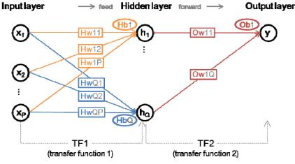
Figure 3. Illustration of typical network model: FFNN.
