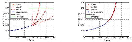
(a) parameters from laboratory tests: prediction set#=8 with biased information
