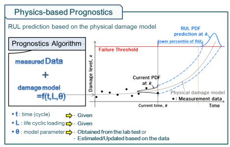
Figure 5. Illustration of physics-based prognostics.
