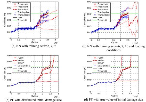
Figure 12. Comparison of NN and PF with the case of complex damage growth under small noise.
