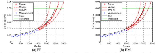
Figure 10. Results from physics-based approaches with the case of simple damage growth under small noise and negative bias.
