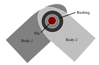
Figure 3: Revolute joint between body-1 and body-2.
