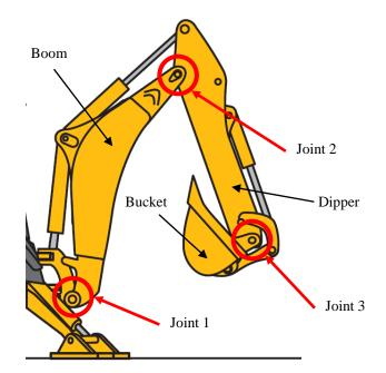
Figure 2: Backhoe system with three main revolute joints.
