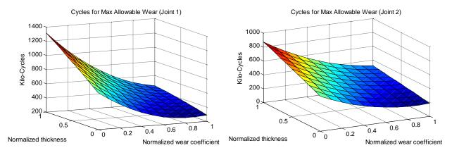
Figure 5: Response generated using the surrogate for  $cyc_1$ .
