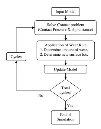
Figure 1: Incremental wear simulation flow chart.
