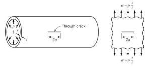
Figure 8: Through the thickness crack illustration
