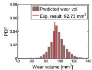
Figure 7: Result of wear volume prediction
