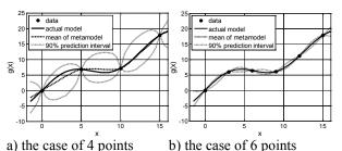
Figure 5: Confidence bands of predictive response function due to the metamodel uncertainty
