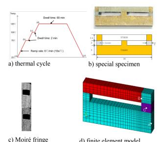
) Moiré fringe d) finite element model Figure 3: Illustrations of creep parameters estimation
