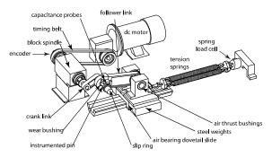
a) the layout of slider-crank mechanism
