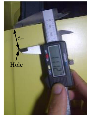
Fig. 6 Edge distance measurement of a fastener hole using a digital caliper.
