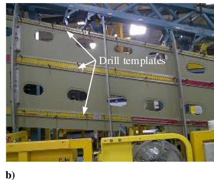
Fig. 5 Representations of drill templates for locating and drilling holes on wing spars.
