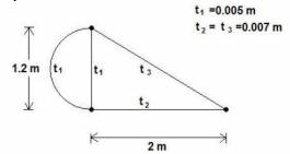
2. A shaft with a channel section shown in the figure is subjected to a torque *T*. Assume that neither end is constrained. Find the warping distribution on the cross-section, the maximum warp, and the location of the maximum warp.
