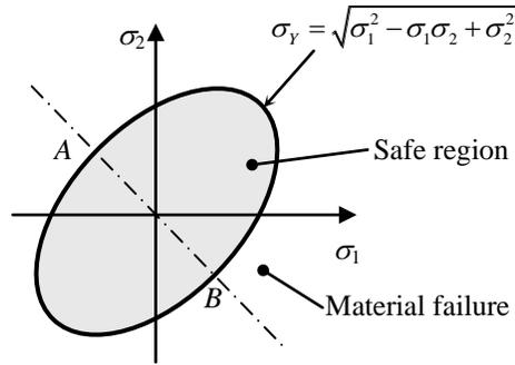
Figure 1.3: Failure envelope of the distortion energy theory
