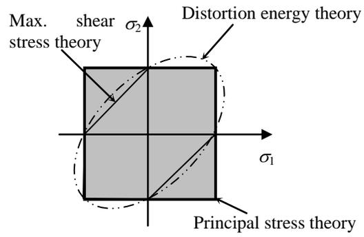
Figure 1.5: Failure envelope of the maximum principal stress theory
