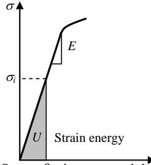
Figure 1.2: Stress-strain curve and the strain energy
