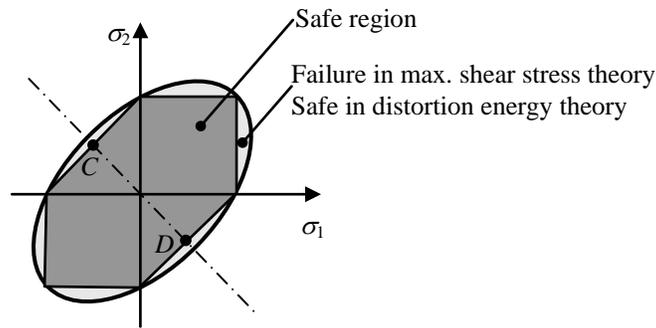
Figure 1.4: Failure envelope of the maximum shear stress theory
