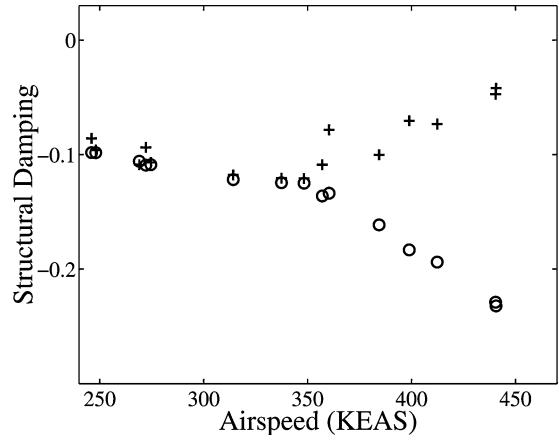
Fig. 2 Measured modal dampings for bending mode, + and torsion mode, ○.
