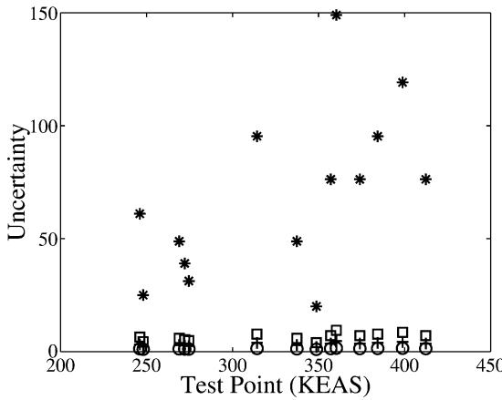
Fig. 9 Uncertainty in updated model for structural stiffness and damping,  $\circ$ ; aerodynamic forces, \*; excitation, +; and measurement,  $\square$ .
