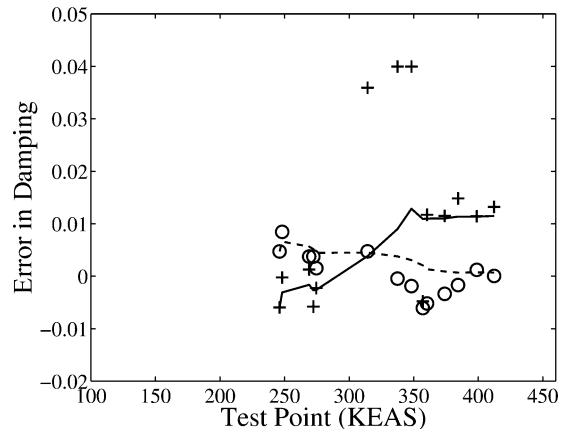
Fig. 6 Error, + and running average of the error, — in modal damping of the theoretical model for bending mode and error, ○ and running average of the error, --- for torsion mode.
