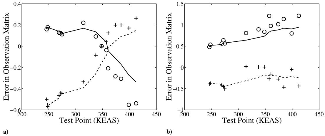
Fig. 8 Error,  $\circ$  and average error, — in observation of first state and error, + and average error, --- in observation of second state of the theoretical model for a) bending mode and b) torsion mode.
