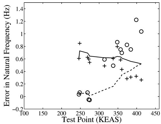
Fig. 7 Error, + and running average of the error, — in natural frequency of the theoretical model for bending mode and error, ○ and running average of the error, --- for torsion mode.
