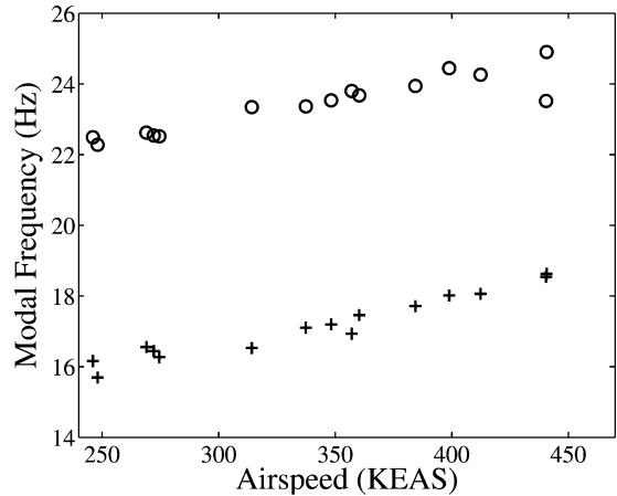
Fig. 3 Measured modal frequencies for bending mode, + and torsion mode, ○.
