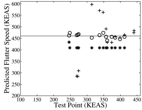
Fig. 10 Flutter speeds predicted by damping extrapolation, +; original flutterometer, \*; and updated flutterometer,  $\circ$ .
