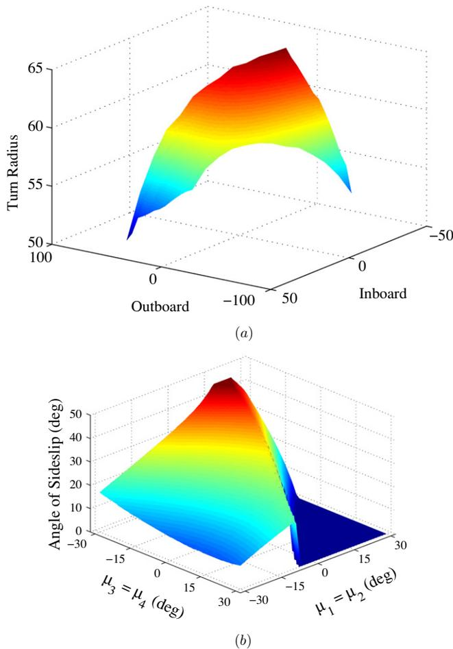
**Figure 5.** Performance of variable wing-sweep aircraft. (a) Turning radius (m). (b) Maximum angle of sideslip at which aircraft can trim.
