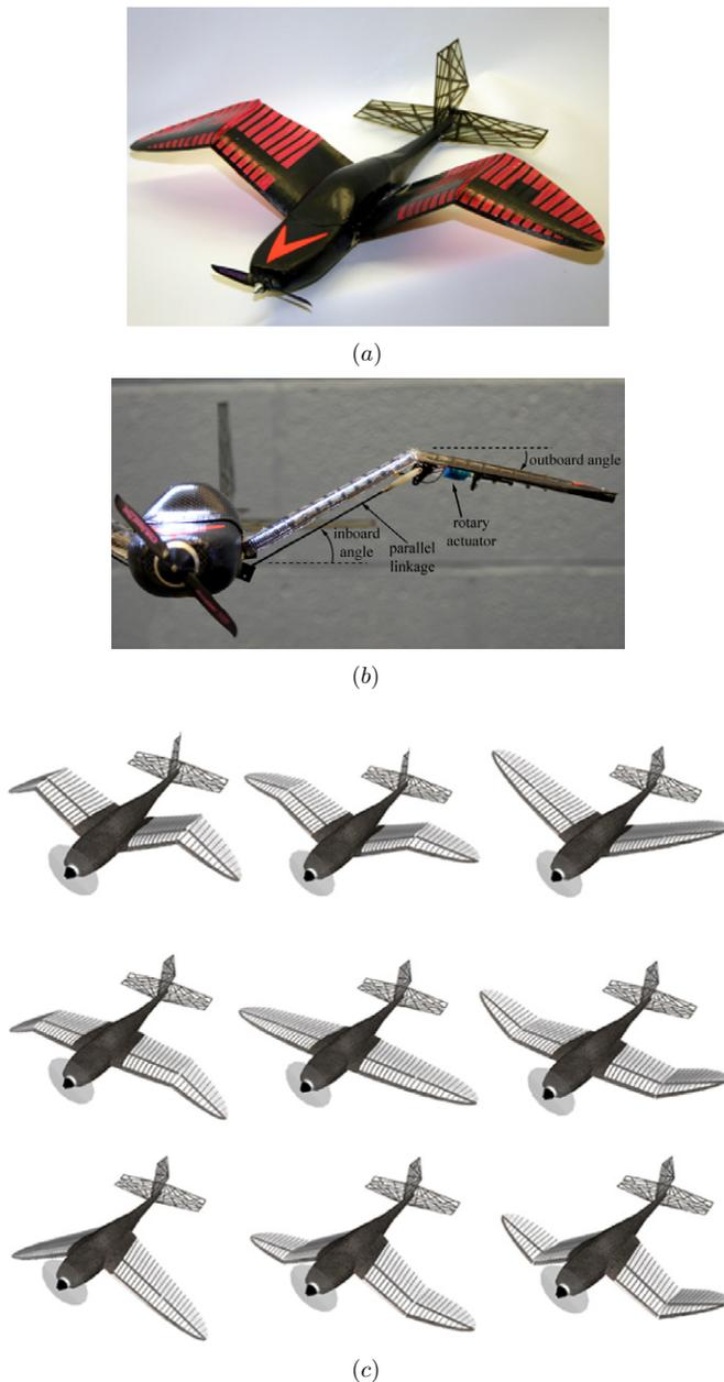
**Figure 2.** Variable gull-wing aircraft. (a) Overview of vehicle. (b) Left wing with an inboard angle of  $\mu_1 = 30^\circ$  and an outboard angle of  $\mu_2 = -12^\circ$ . (c) Range of configurations.
