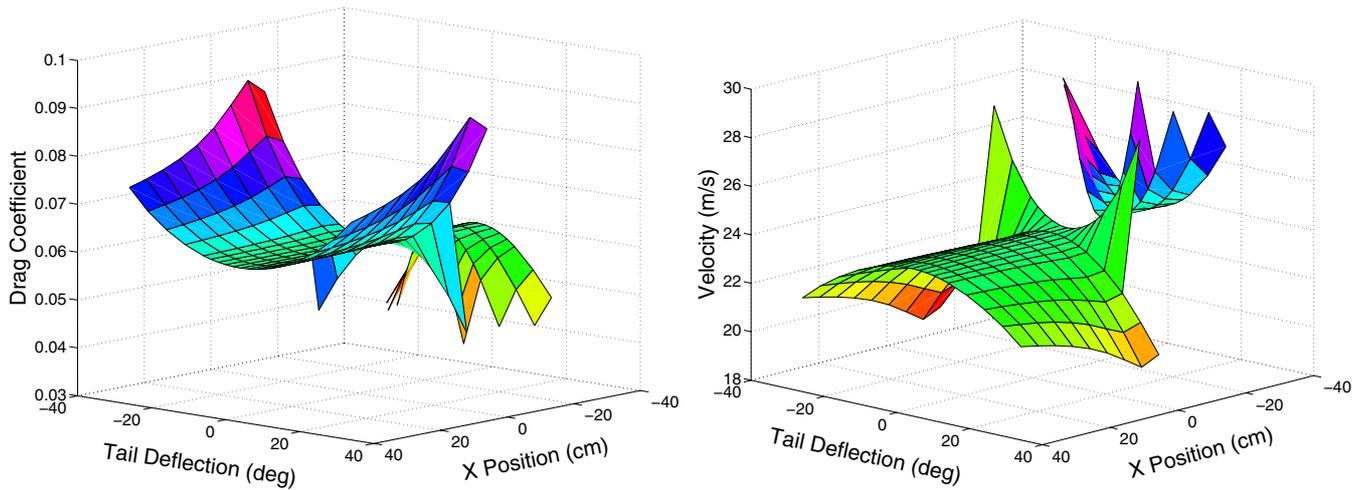
Figure 14. Drag coefficient and trim velocity in a 45° banked turn.
