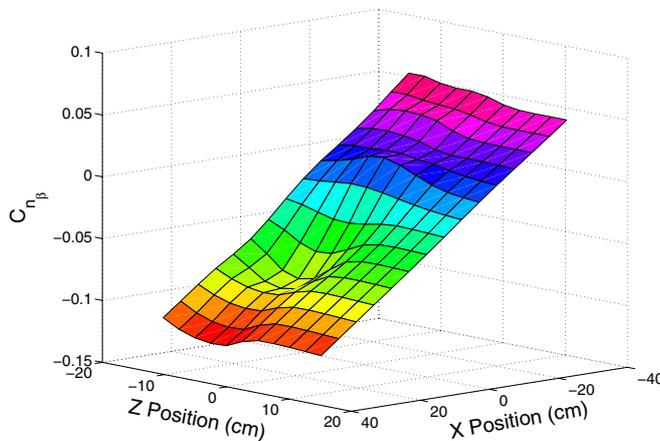
**Figure 6.** Yaw moment coefficient with respect to the angle of sideslip for straight-and-level flight.
