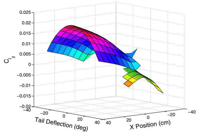
**Figure 12.** Roll moment coefficient with respect to the angle of sideslip in a 45° banked turn.
