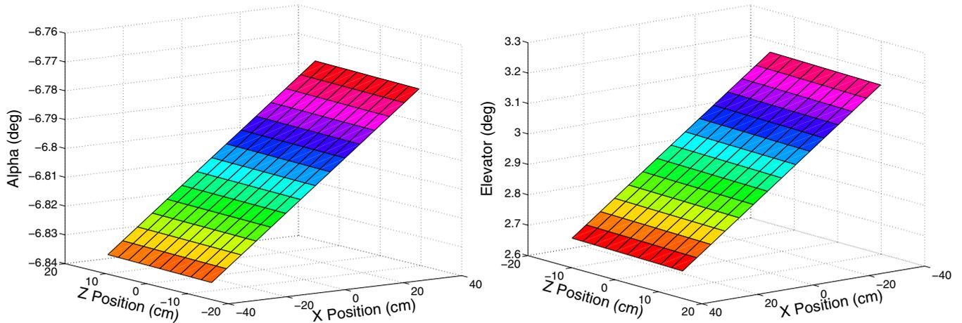
**Figure 4.** Trim for straight-and-level flight: angle of attack (left) and elevator deflection (right).
