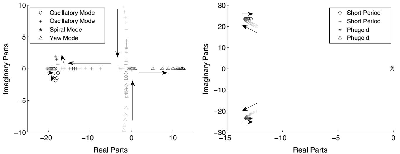
Figure 15. Eigenvalues as the vertical tail moves forward: lateral-directional (left) and longitudinal (right).
