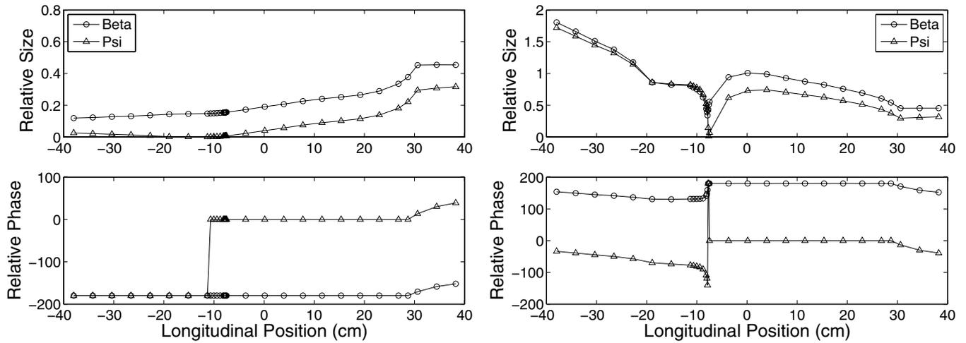
**Figure 16.** Eigenvectors for variations in the longitudinal location of the vertical tail for eigenvalue associated with aft-location roll convergence (left) and aft-location Dutch-roll mode (right) with a normalized roll angle.
