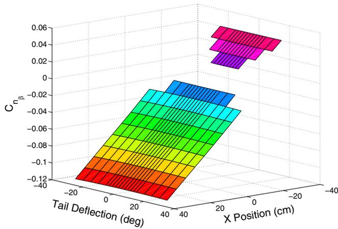
**Figure 11.** Yaw moment coefficient with respect to the angle of sideslip in a 45° banked turn.
