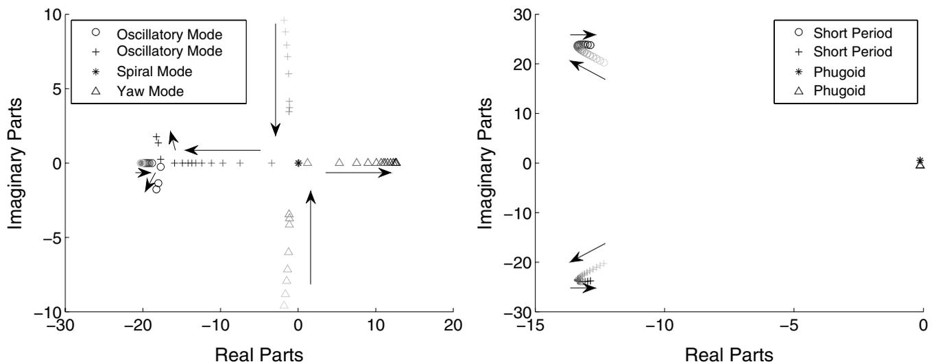
**Figure 19.** Turning mode eigenvalues as the vertical tail moves forward: lateral (left) and longitudinal (right).
