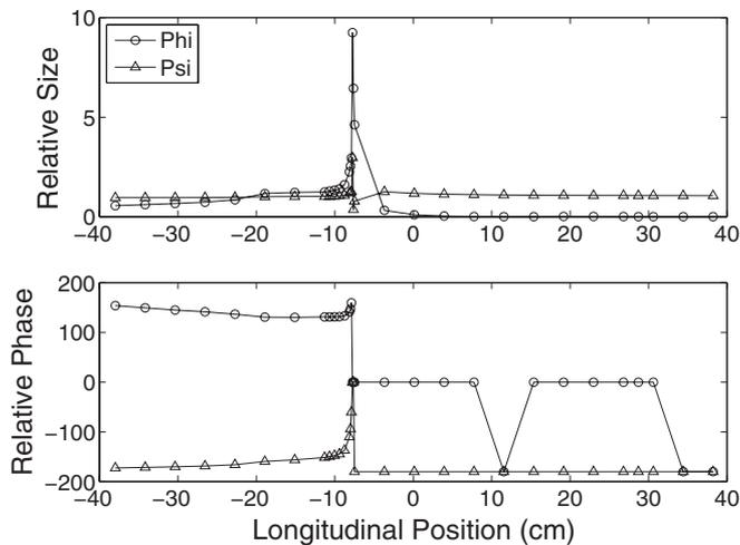
**Figure 17.** Eigenvectors for variations in the longitudinal location of the vertical tail for eigenvalue associated with aft-location Dutch-roll mode with a normalized angle of sideslip.
