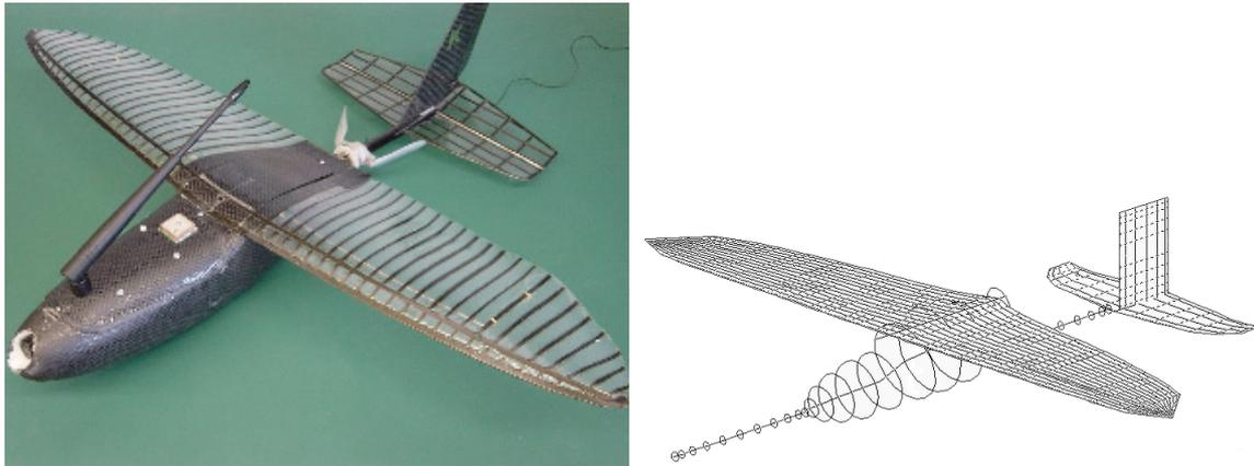
**Figure 2.** Existing aircraft (left) and baseline shape for pterosaur-inspired vehicle (right).
