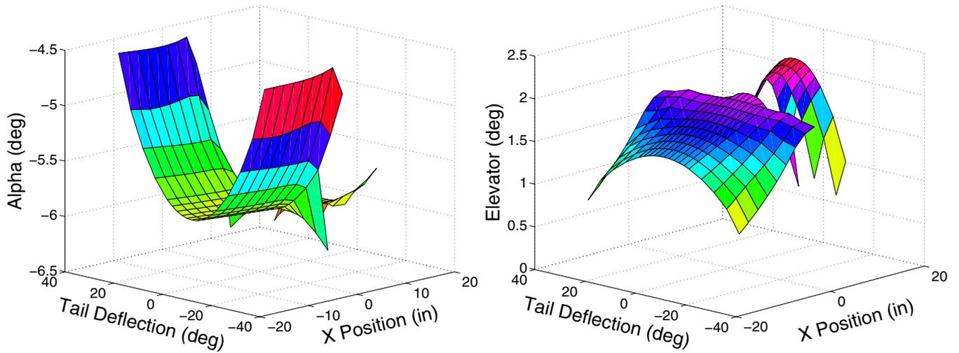
Figure 8. Trim in a 45° banked turn: angle of attack (left) and elevator deflection (right).
