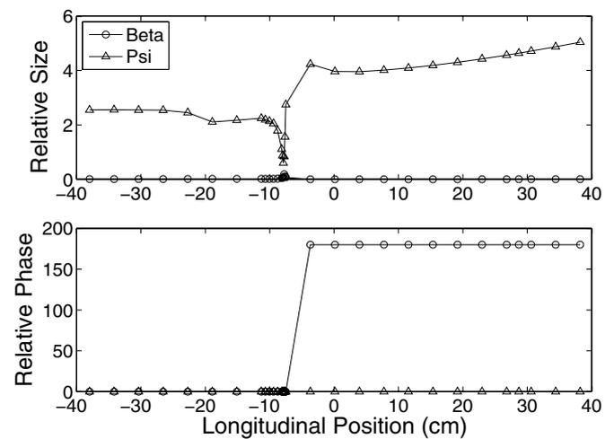
**Figure 18.** Eigenvectors for variations in the longitudinal location of the vertical tail for eigenvalue associated with aft-location spiral divergence with a normalized roll angle.
