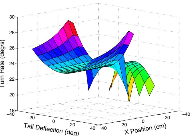
**Figure 13.** Turning metrics in a 45° banked turn with respect to vertical tail deflection and longitudinal placement.
