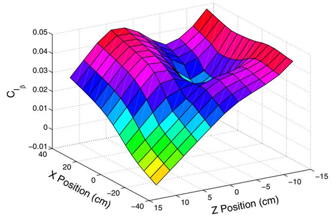
**Figure 7.** Roll moment coefficient with respect to the angle of sideslip for straight-and-level flight.
