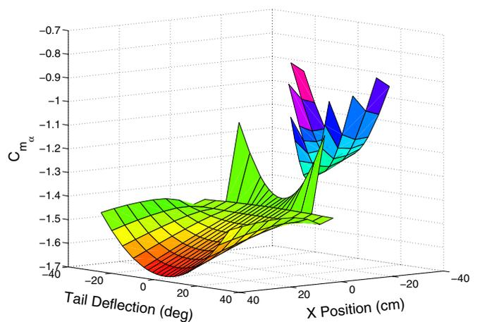
Figure 10. Pitch moment coefficient with respect to the angle of attack in a 45° banked turn.
