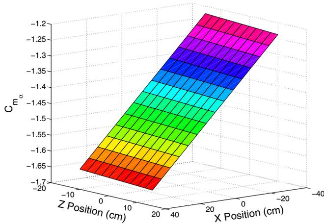
**Figure 5.** Pitch moment coefficient with respect to the angle of attack for straight-and-level flight.
