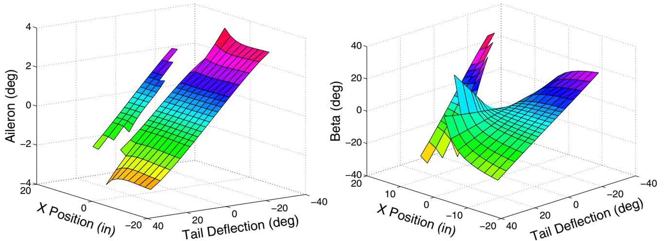
Figure 9. Aileron deflection and angle of sideslip in a 45° banked turn.
