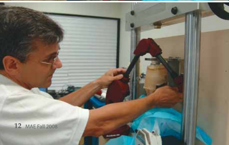
B.J. Fregly works on a cadaver knee wear experiment to simulate the arthritis process at Scripps Clinic in La Jolla, CA. This work is the first step toward the human subject simulations that will be performed in the current research project.
