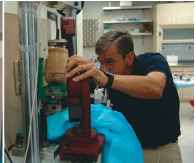
B.J. Fregly works on a cadaver knee wear experiment to simulate the arthritis process at Scripps Clinic in La Jolla, CA. This work is the first step toward the human subject simulations that will be performed in the current research project.
