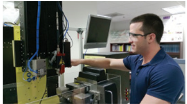
Paul Moore (UF-PhD student) uses a dual axis Sarix 200 3D \mu EDM/ \mu -milling machine for fabricating a prototype middle ear prosthesis, working with Francesco Modica (ITIA-researcher).
