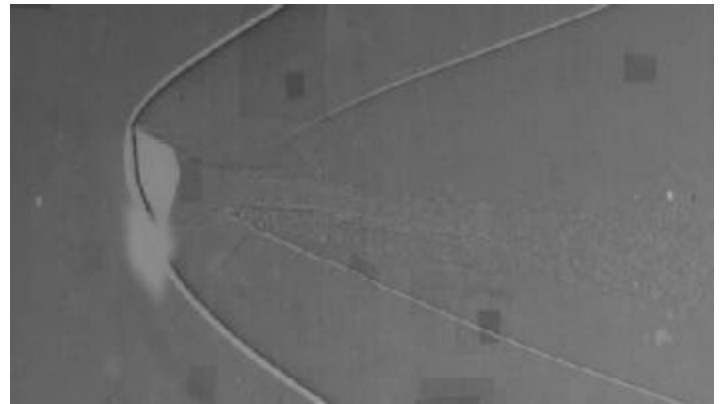
Shadowgraph of the Mars Explorer Rover Mission lander entry capsule flying in the ARF
