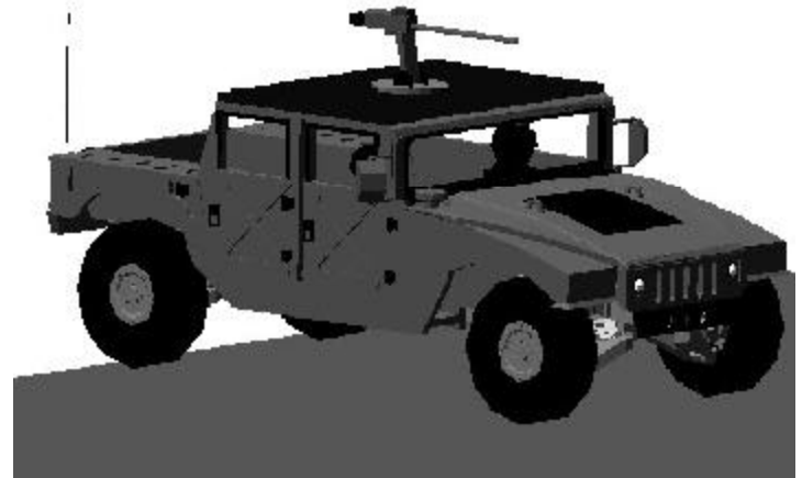
Figure (3) Nonlinear multibody model of high mobility vehicle with weapon platform. Developed in conjunction with Dr. Mike Hale, Redstone Arsenal.
