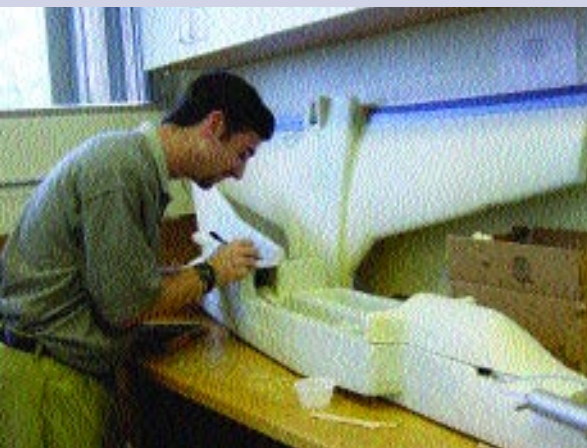
Mujahid Abdulrahim with his prototype morphing aircraft. This 6-foot wingspan aircraft has a segmented morphing trailing edge surface.
