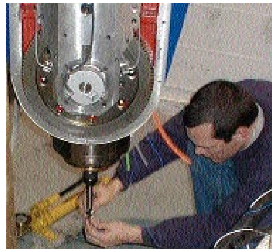
Tony Schmitz attaching accelerometer to cutting tool (mounted in high-speed spindle) in preparation for frequency response measurements.
