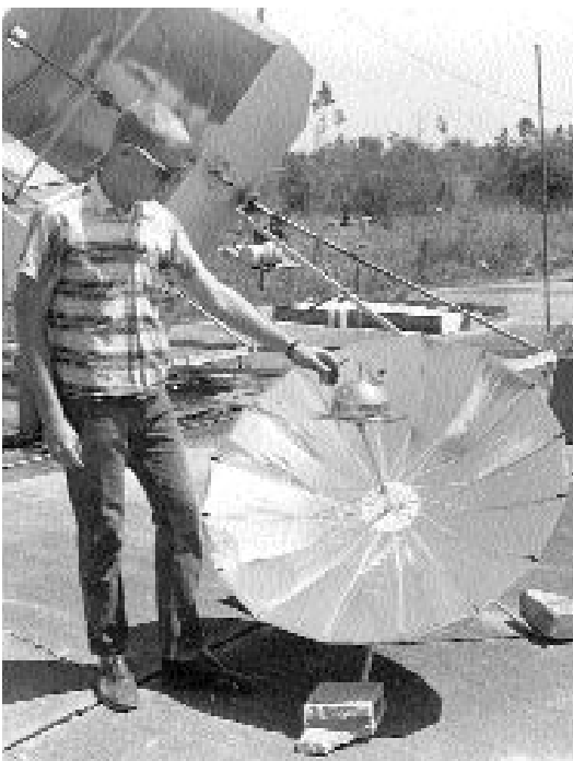
(TOP) Early SEECL student demonstrates solar cooking on a collapsible umbrella cooker. The concentrated solar radiation heated the teapot quite effectively – and the collapsing umbrella made storage easy (mid 1950s).
