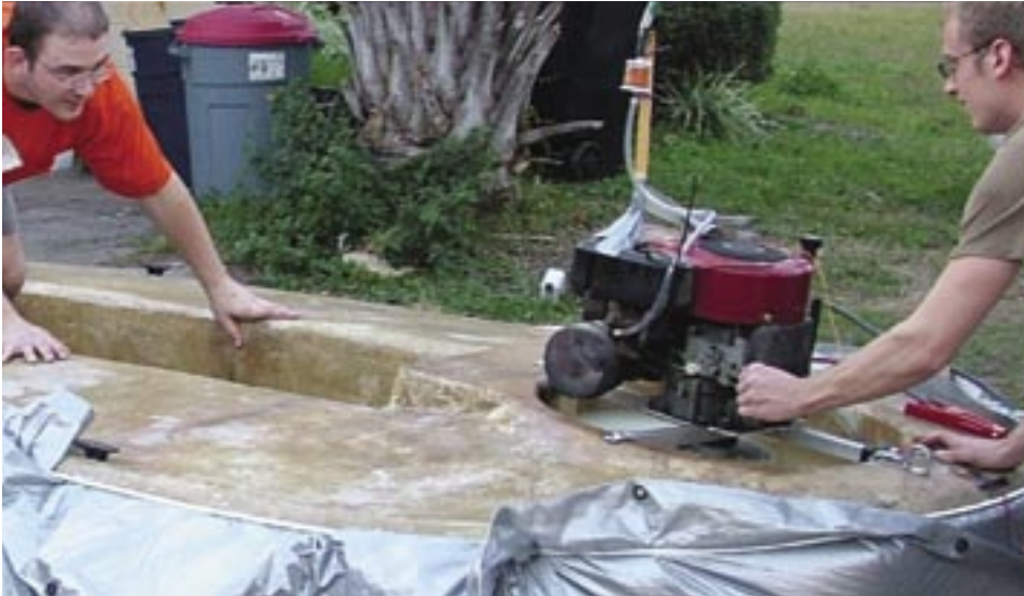
(L-R) Doug Jones and Tim Bernhard conducting a lift test, using a bag skirt
