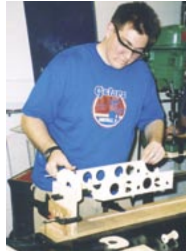
Tristan Goldbach is mounting a longeron onto a fuselage
