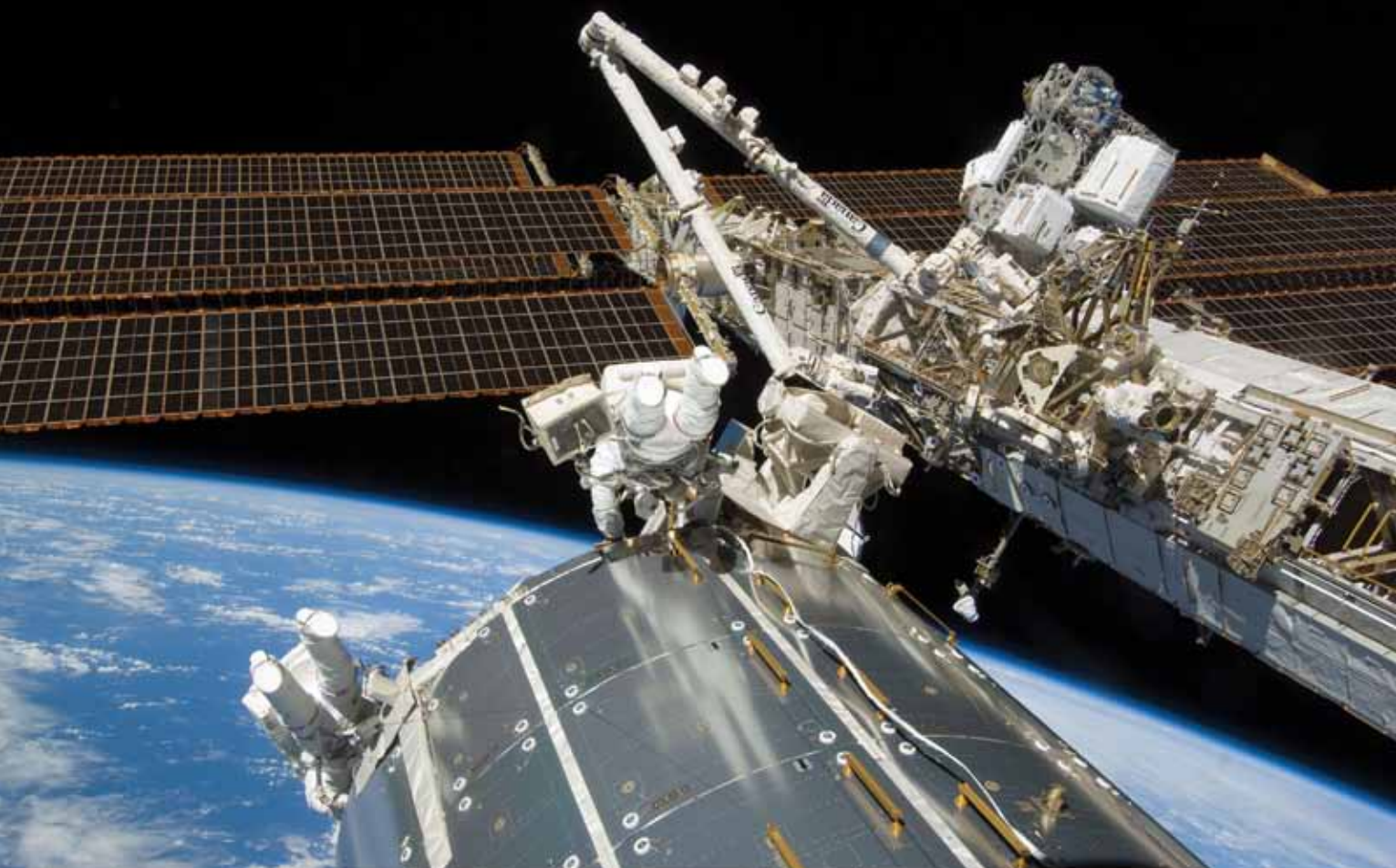
STS-129 Astronauts on a space walk. During the third space walk the MISSE 7 experiments were installed and turned on. All 8 tribometers successfully turned on and began making measurements in space. On the top right of the image the Express Logistics Carrier can be seen attached to the ISS.
