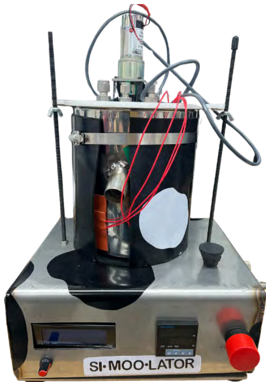
The Si-Moo-Lator™ was designed with cleaning accessibility in mind using a easily scrubbed steel vessel to avoid cross contamination between experiments.
