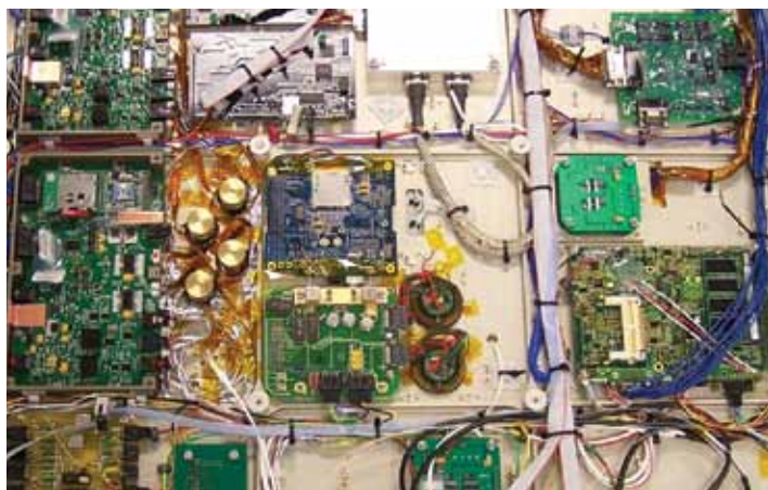
5 The experiment control electronics mounted to the bottom side of the baseplate directly beneath the experiments.
