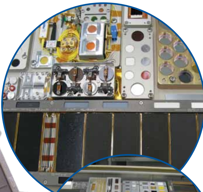
7 The “wake” tribometers mounted in the MISSE 7 PEC with all the other MISSE experiments. The wake side of the ISS faces the direction opposite the ram. This side experiences Ultra High Vacuum (UHV).
