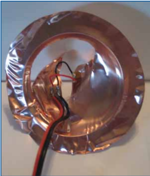
A burst copper disc with strain-gage still attached.
