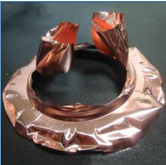
A burst copper disc after rupture.
