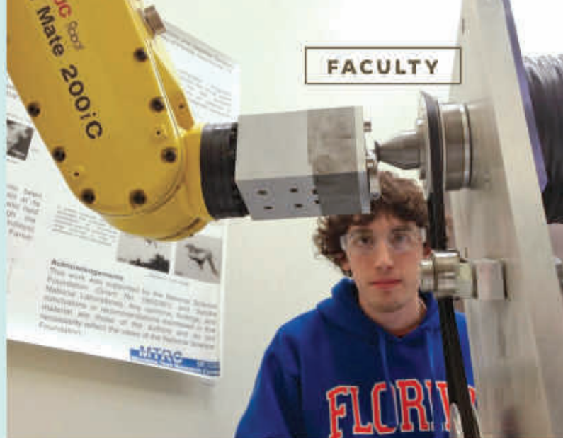
MAE graduate student Max Stein runs a polishing experiment using a six-axis robot for the Zeeko project.
