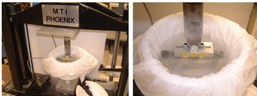
Fig. 12. Cryogenic experimental setup of the four-point bending test.
