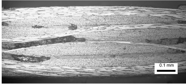
Fig. 10. Cross-sectional view of the woven composite specimen T1 before cryogenic cycling, 10 \times magnification.
