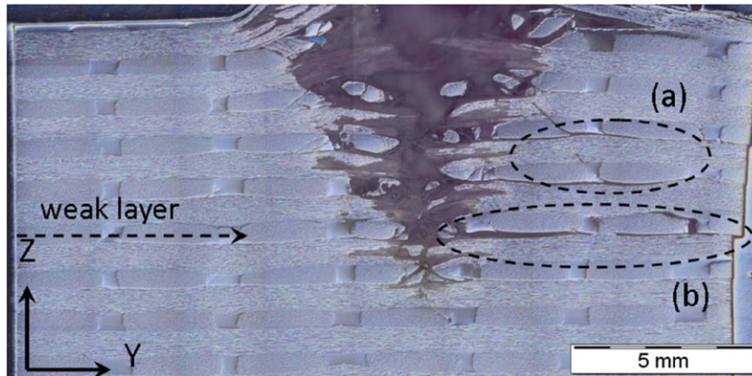
Fig. 6. Cross-section along y – z plane showing damage due to intermediate indentation depth. (a) Small delaminations arrested by z -yarn, and (b) large delamination along weak layer.
