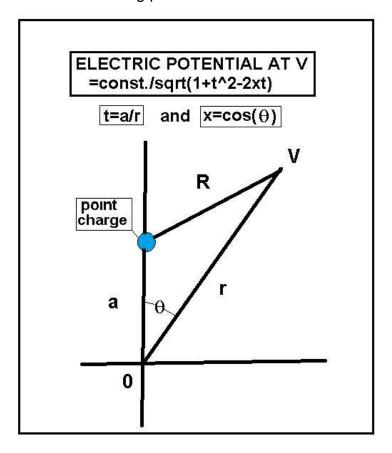
The potential at V from this point charge goes as const/R. Using the Law of Cosines and setting any common const to unity, the potential at V is-
