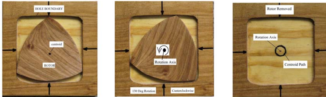
WOOD MODEL OF MOVABLE REULEAUX TRIANGLE FOR DRILLING NEARLY SQUARE HOLES
