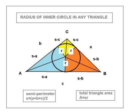
Next we bisect the angles A, B, and C with straight lines heading toward a common center which is the location of the centroid of the triangle. At this centroid a circle of radius r which just touches the triangle boundaries can be drawn. This represents the desired inscribed circle in the triangle. Some simple arithmetic now gives the entire triangle area as –
