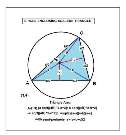
We next draw three redlines perpendicular to the center points of the three triangle sides. These meet at a common center point which defines the center of a new circle. Note that the circle center lies at coordinates –
